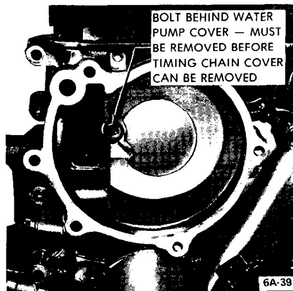
Figure 6A-39 Bolt Behind Water Pump
