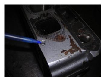
I also drill out the plug that's on the face of the head, below the #1 exhaust manifold attachment bolt. It's the intersection passage for the oiling to the head. Lots of grit tends to accumulate there after a trip to the machine shop! This needs to be drilled out oversize, and I use a 1/8" NPT plug there.
