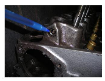
For the main gallery, 1/4" NPT works perfectly without drilling out the holes but be aware that you must use either a shorter forward pipe plug OR don't tap the hole as deeply up front. If you go too far in with a plug, you will block the oil flow from the forward cam bearing to the rest of the head, with disastrous results...
