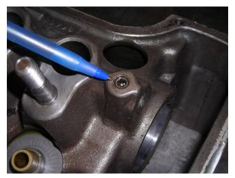
Cam bearing oil feed holes are originally fitted with aluminum plugs. Early heads have three of these, while later heads (late 1970/early 1971) have four of these. I tap these for an 8mm x 1.00 metric pipe plug.
