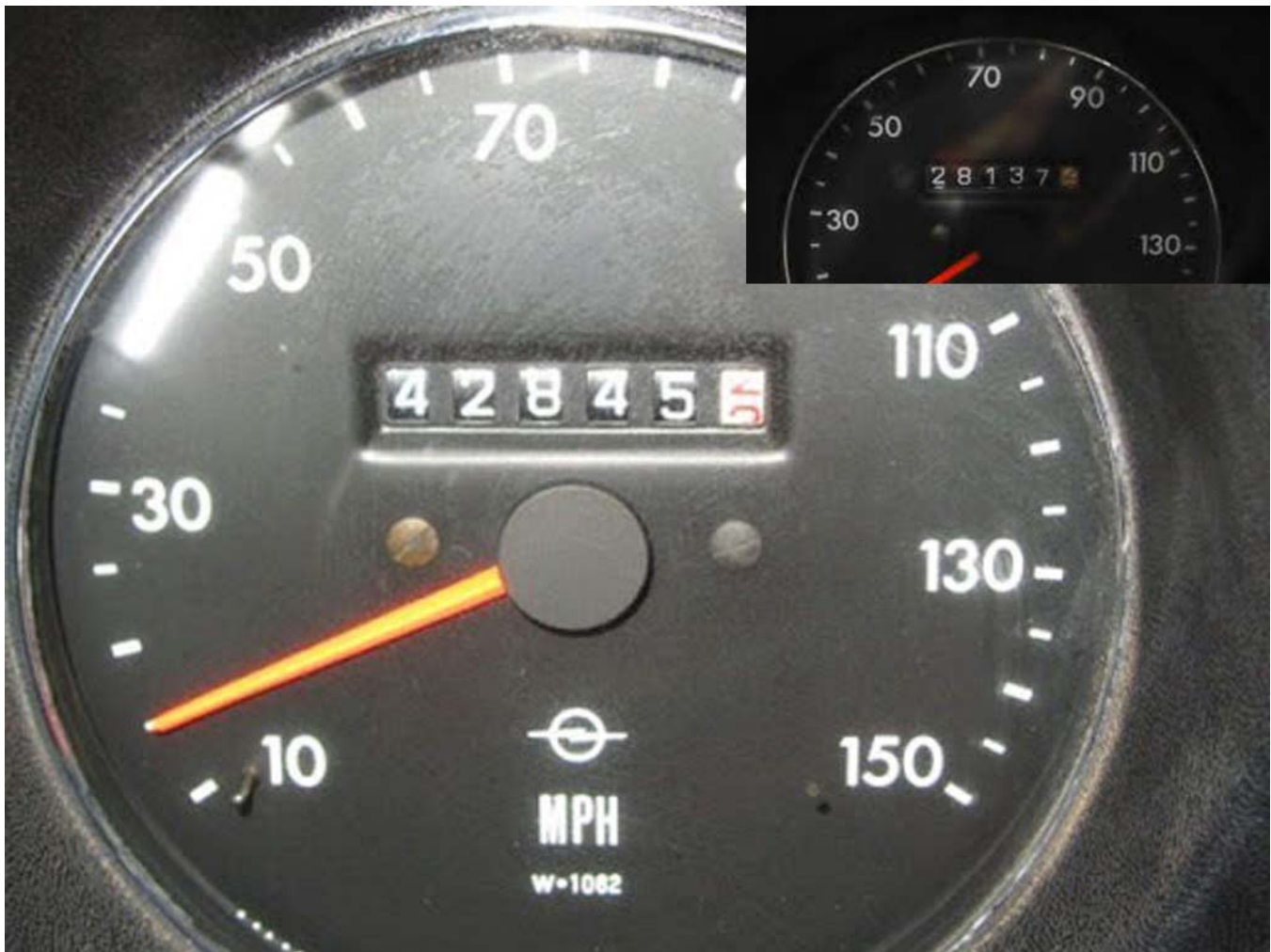
This odometer has not flipped, has not passed 99,999 miles. The one in the top right has. The tell tale sign is the numbers are not centered vertically in the opening.
